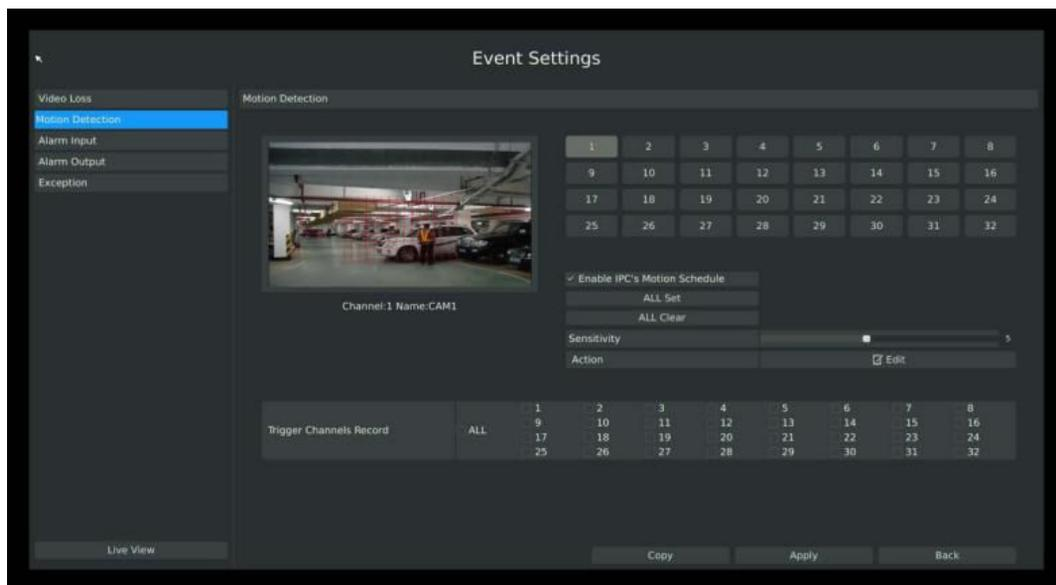
Figure 1.1 Motion Detection Settings in Local Monitor
