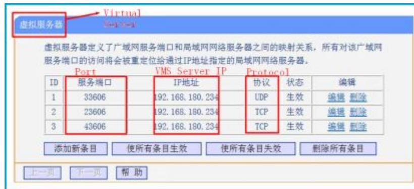
For specific ports you should use corresponding protocols. Like 23606→TCP, only TCP will be allowed in database port 23606.
